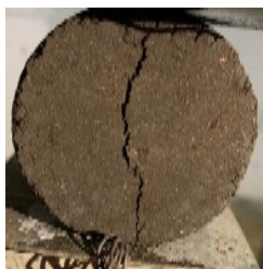
(a) vertical crack
