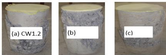
Fig 4: Crack Mode and Collapse of Confinement Wire Mesh
